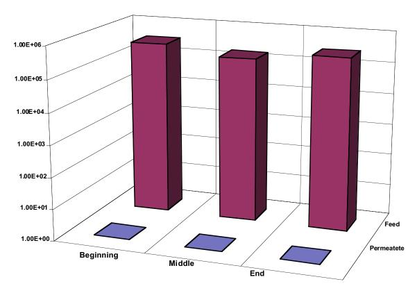
Virus rejection by Hydranautics capillary UF membranes. High fouling conditions.
