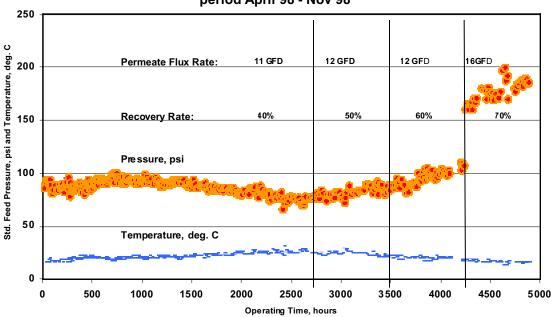
Figure 17-SAN PASQUAL SITE Wastewater Effluent, Capillary UF Pretreatment LFC1 Membrane Elements, Apr98 to Nov98
